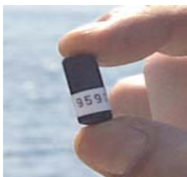
Figure 7.3 The acoustic transmitter (V8SC) used to detect Australian bass in proximity to a VR2 listening station.
